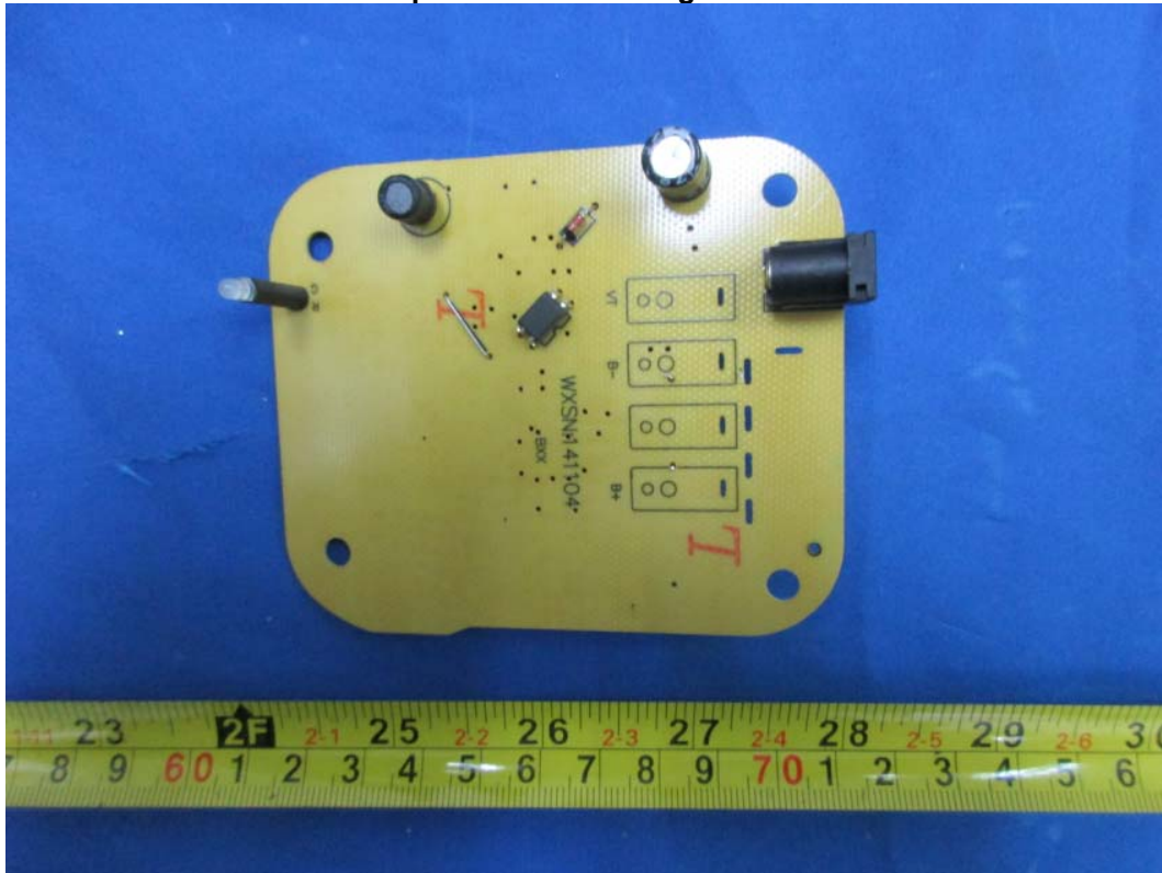
Bottom PCB view of charger base
